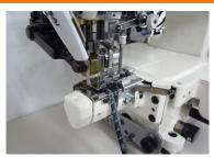
Equipped with an exterior looper thread take-up cam, it is easy to thread and adjust. The automatic thread trimmer increases productivity.
