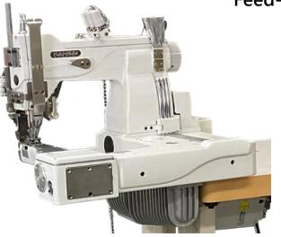
Feed-off-the-arm machine for tape attaching
