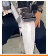
This model is equipped differential feed dog mechanism.
