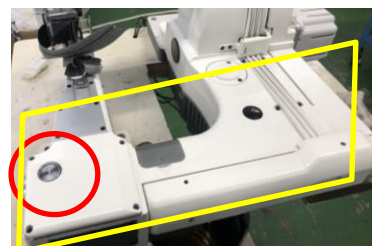
Push button stitch length adjustment
