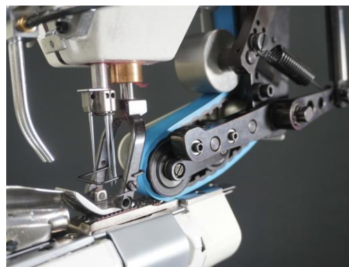
Differential feed mechanism 2 kinds of feed dogs are included in the machine
