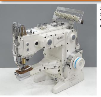
2-needle, 4-thread feed-up-the-arm double chain stitch machine for attaching tape to cover the overlock seams on shoulders and the back of the neck of T-shirts and Polo shirts
