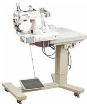
The "-DG" model, which will also be exhibited at the exhibition, is equipped with a patented independent needle guard mechanism in Japan. Which is three needle square type of feed-off-the-arm, double chain stitch machine.
