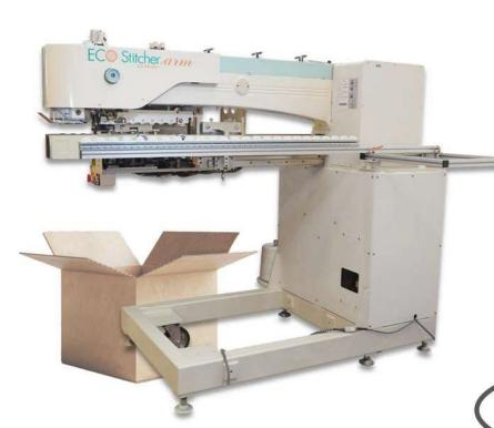
Cardboard sewn with the Eco Stitcher has passed abrasion resistance tests (thread and liner) of 4,000 times, and compression and peel tests have confirmed that it is stronger than wire joints.
