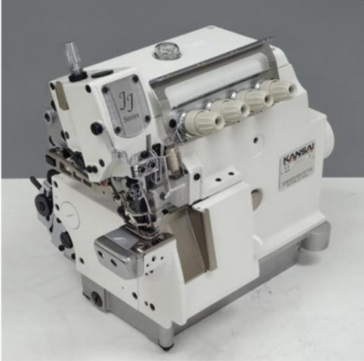
2 needles 4 threads overlock with 148mm circumference cylinder.
